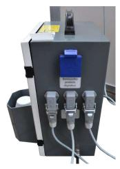
Switch the key switch on the front of the control unit to the "I" position. The positive locking control is now active.
