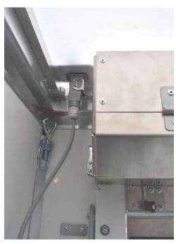
Connect the supplied electrical cables to the three connections on the outside of the roof (where the plugs are also connected from the inside) and connect them to the forced locking control unit. It does not matter in which order the three plugs are connected to the control unit.
