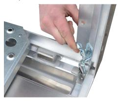
Insert the roller shutter guide and wall panel into the mounting brackets of the floor panel and the corner profile. Secure the roller shutter guide with wing screws / wing nuts.
