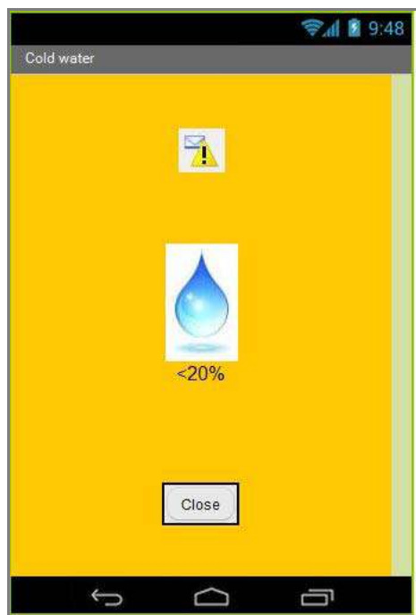
Fig. 1 120 Warning message Filling level of cold water tank below 20%
