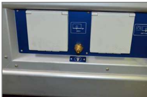
Fig. 1 124 Compressed air feed
