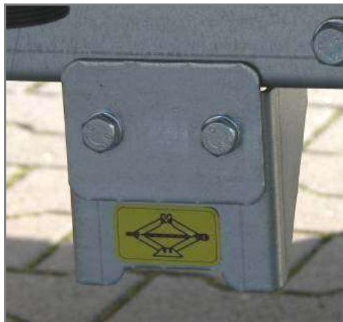
Fig. 1 22 Contact points for the jack
