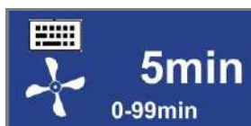
Fig. 1 46 Setting of the time for which the negative pressure unit continues to run after all persons have left the decon unit
